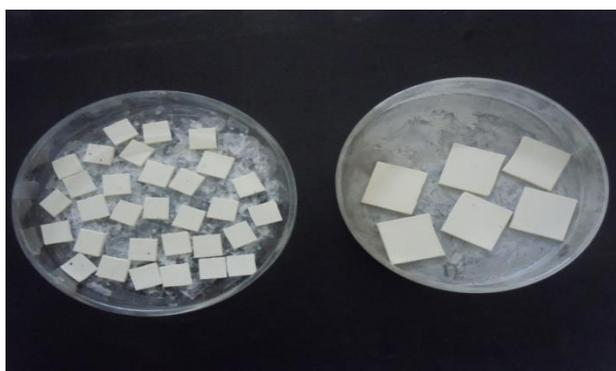
**Figure 2.4: TiO<sub>2</sub> coated chips for analysis**
