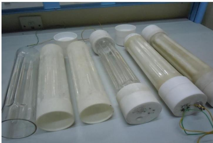
**Figure 2.1: TiO<sub>2</sub> coated reactors with teflon caps**
