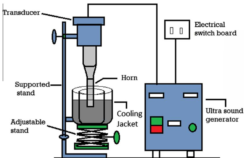
Fig. 3. Experimental setup for synthesis of undoped and doped TiO<sub>2</sub> nanoparticles.
