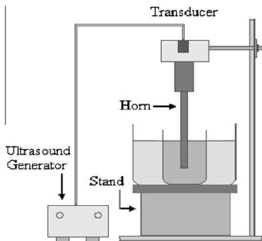
Fig. 2. Experimental setup for sonochemical synthesis.
