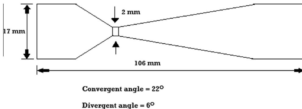
Fig. 2. Geometrical dimensions of cavitating device (circular venturi).
