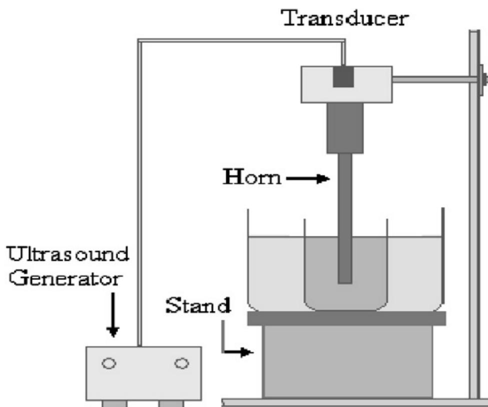
**Fig.4.** Experimental set up for sonochemical synthesis of nanoparticles [Reprinted from (8).
