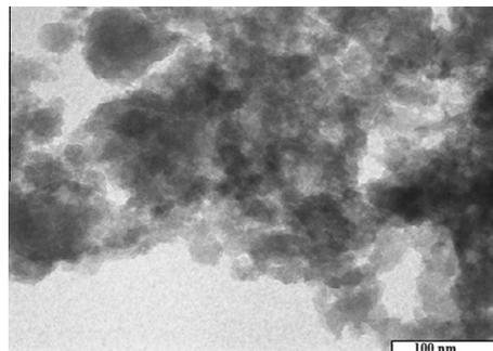
Fig. 8. TEM image of 1.6 mol% of Ce doped-TiO<sub>2</sub>.
