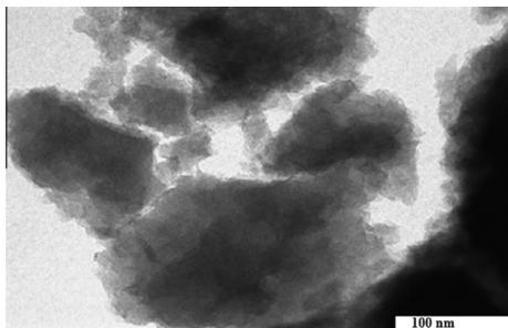
Fig. 6. TEM image of pure TiO<sub>2</sub>.
