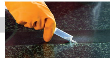
6b Collect mercury droplets using syringe
