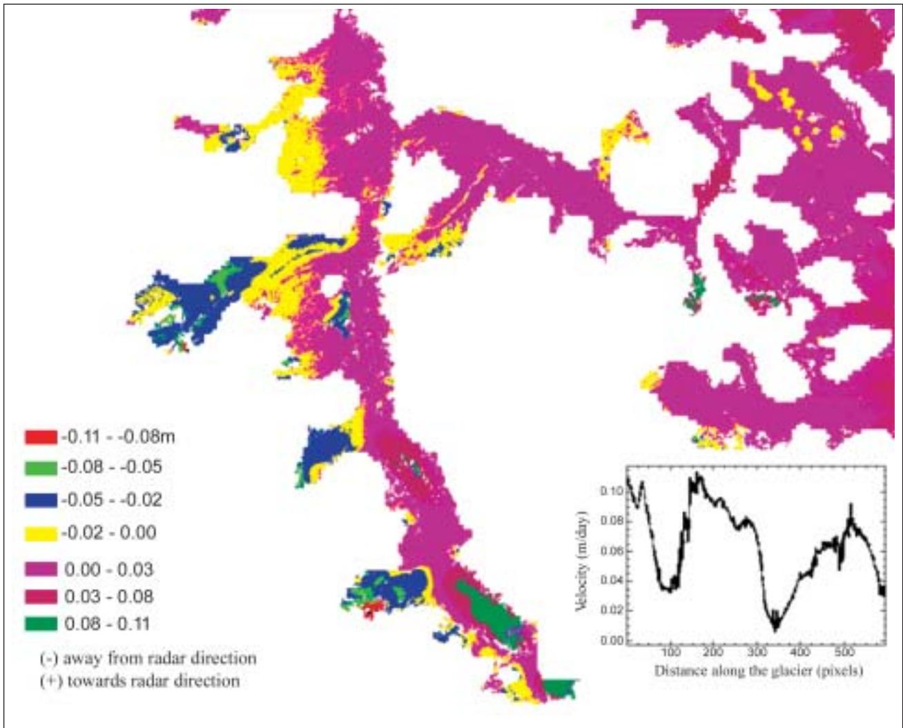
Fig. 20: Plot of velocity in the radar direction for ascending pass over Gangotri glacier.
