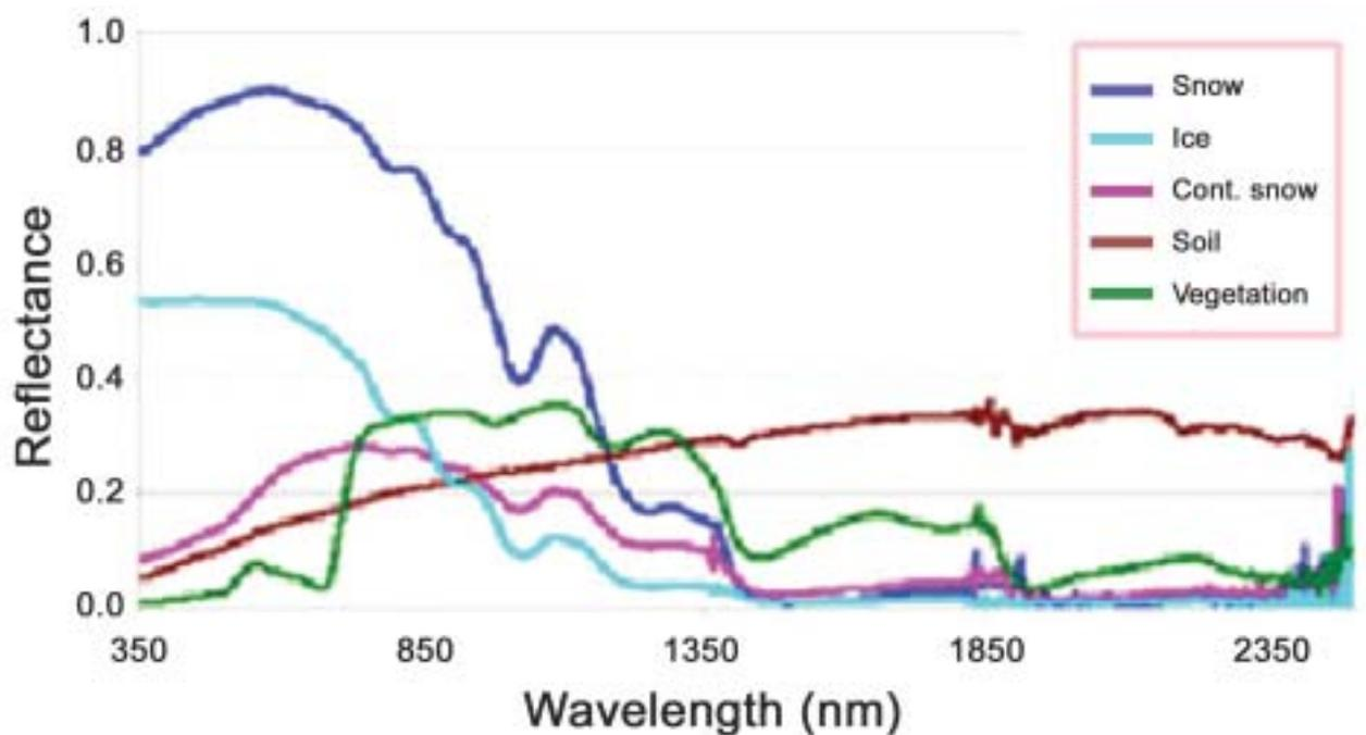
**Fig. 24:** Spectral reflectance of snow, ice, contaminated snow, vegetation, and soil. observations taken using spectral radiometer near Manali, H.P.
