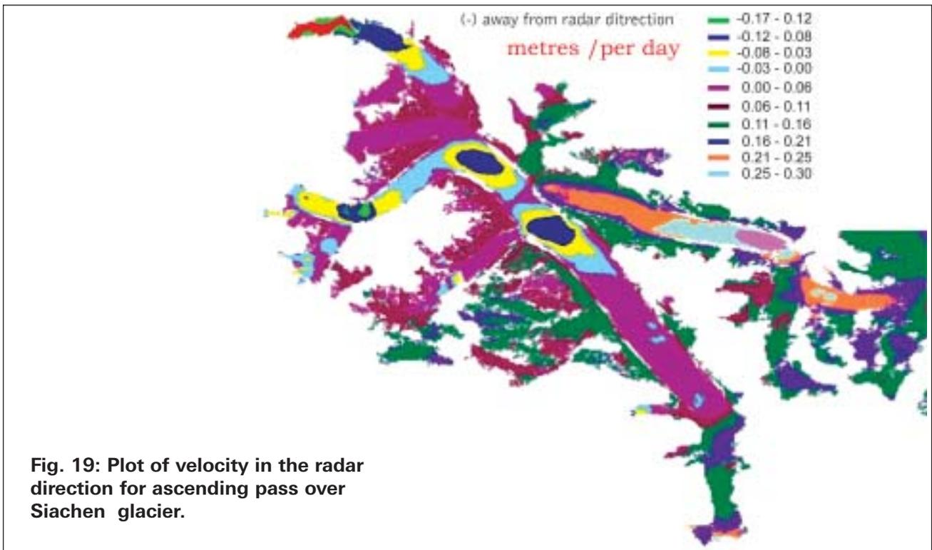
**Fig. 19: Plot of velocity in the radar direction for ascending pass over Siachen glacier.**
