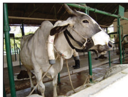
Figure 2.18: Estimation of enteric methane emission from cattle using \text{SF}_6 tracer technique
