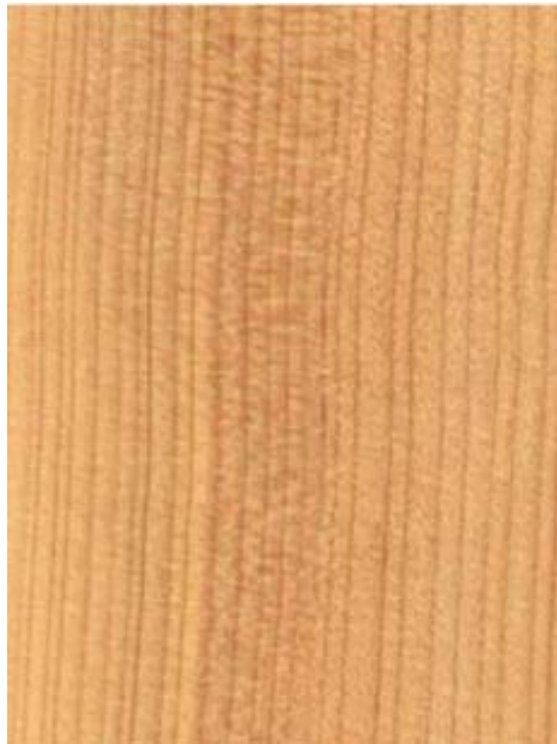
Fig-36. Face veneer produced from reconstituted flitch.
