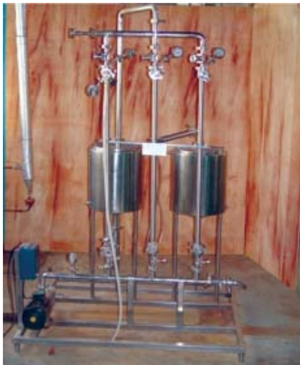
Fig-27. Ultra filtration for molecular fractionation of lignin in black liquor
