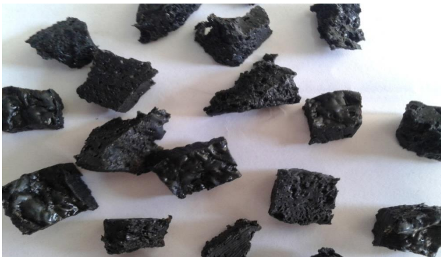
Fig.34. Ultrasonically prepared PAA-GO nanocomposite hydrogel
