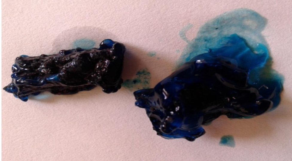
Fig.29. MG adsorbed PAA hydrogel beads
