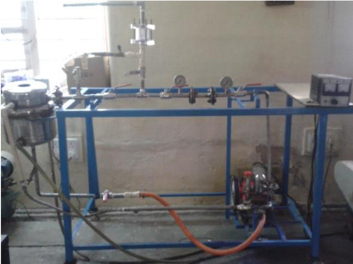
Fig.26. Hydrodynamic cavitation+Hydrogel packed bed (hybrid system)
