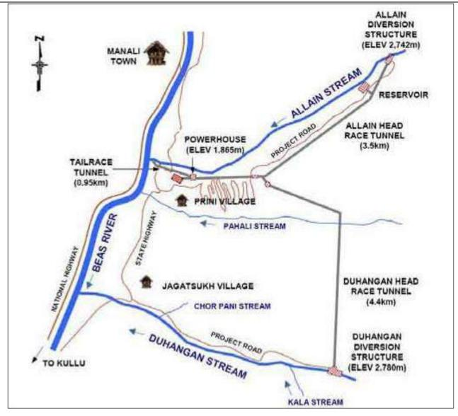
Figure 2.2: Layout Plan of Allain Duhangan HEP
