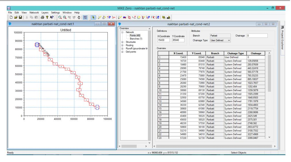
Figure 8.1: Location of various surveyed river cross sections (A typical MIKE 11 model set-up)
