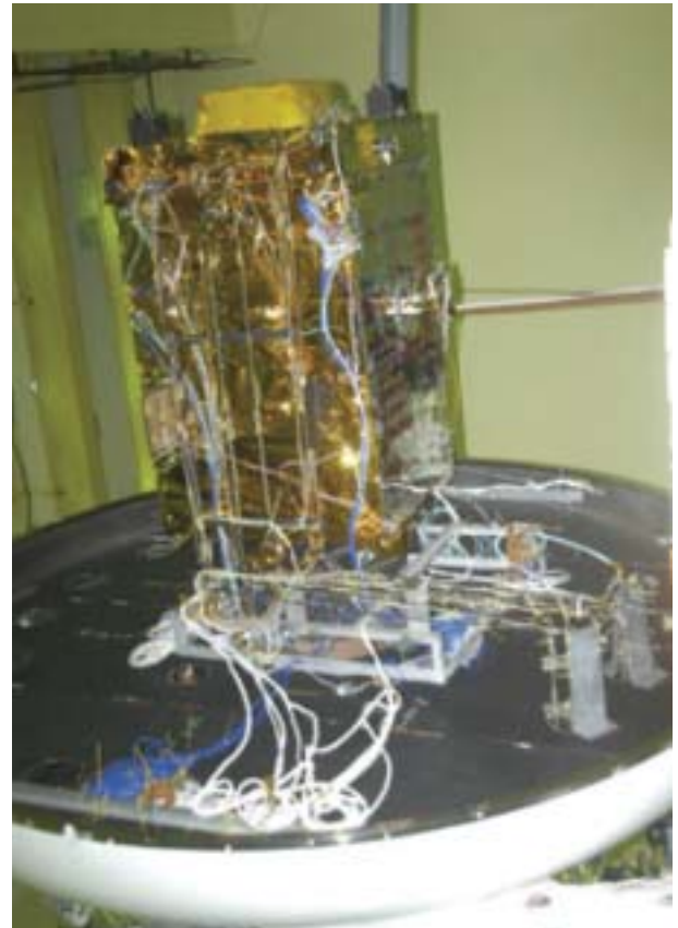
GSAT-4 ready to enter CATVAC
