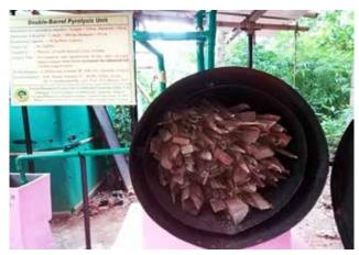
Double-Barrel Pyrolysis System
