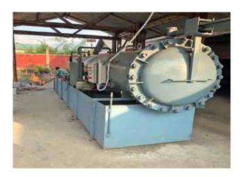
Four number of Vacuum pressure treatment units were established in Manipur at four location viz., Sowmbung, churachandpur, Khangsim and Noney. At Sowmbung a Vacuum pressure treatment unit -22 feet length and 3.3 feet diameter was installed and at other three locations
