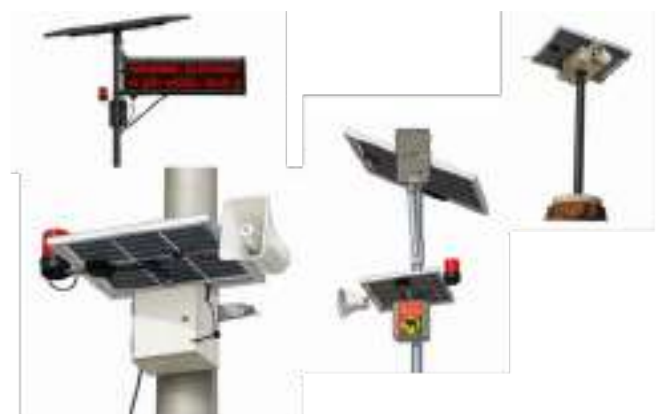
Figure 6. GSM and App based hooters used in Dhenkanal Forest Division; 3a) GSM hooter with streetlight, 3b) Portable GSM hooter, 3c) GSM hooter with LED panel, 3d) App based hooter.
